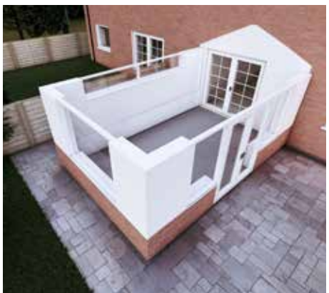
New frames and hup! walls on cill.
